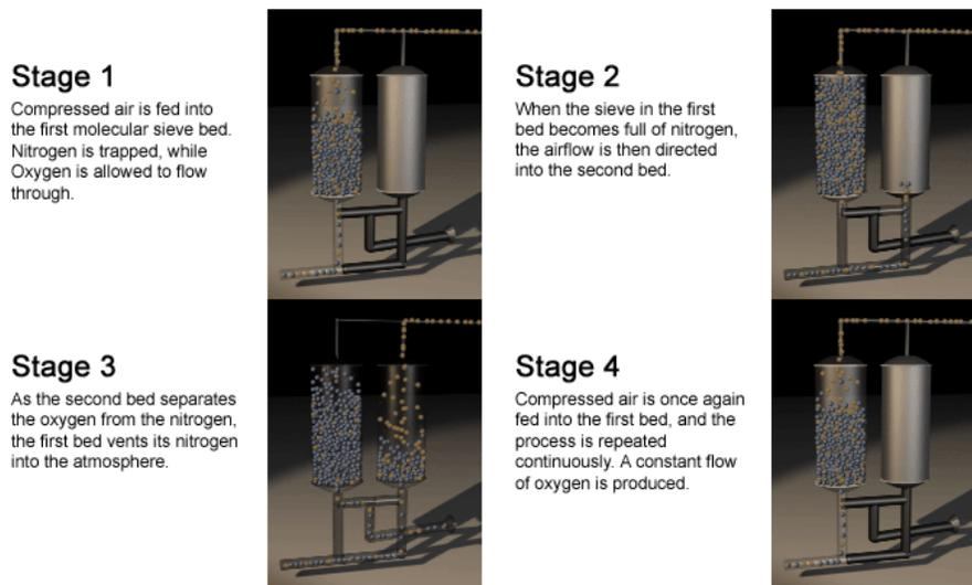
**Figure 2.2 Pressure Swing Adsorption Process (16)**
