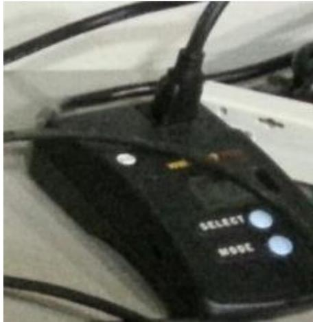
**Figure 3.9 Watts Up Power Meter**
