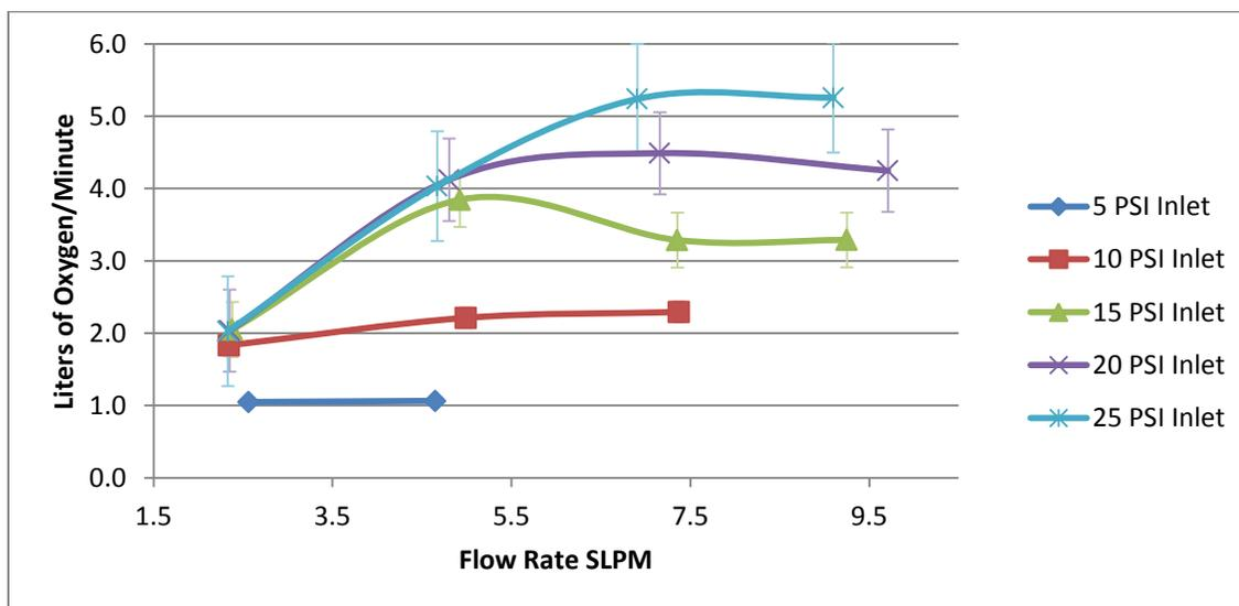
**Figure 5.9 Variable Inlet Pressure Oxygen Flow Rate**
