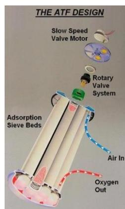
**Figure 5.13 Exploded Diagram of the Sequal ATF System (21)**
