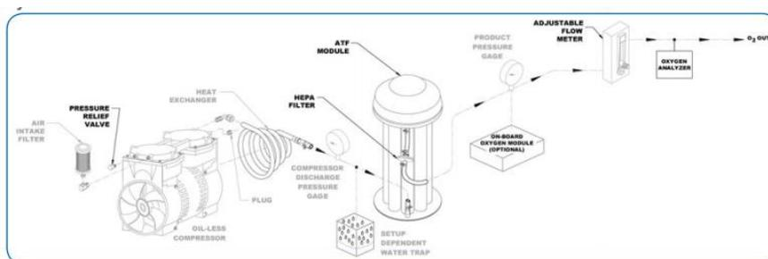
**Figure 5.11 Exploded Diagram of the Sequal Workhorse System (22)**
