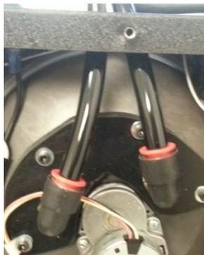
**Figure 4.4 Added Exhaust Plate and Hosing**
