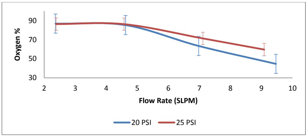
**Figure 6.1 Oxygen % Versus Flow Rate at 20 and 25 PSI**
