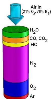
**Figure 5.17 ATF Column Zeolite Structure (21)**
