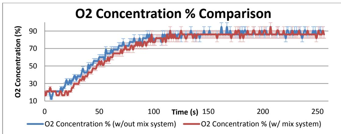
**Figure 4.6 Oxygen % Comparison With and Without the Added Plate**
