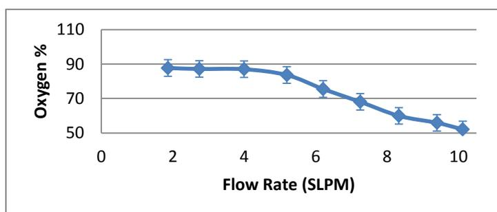
**Figure 5.1 System Oxygen % Versus Output Flow Rate**
