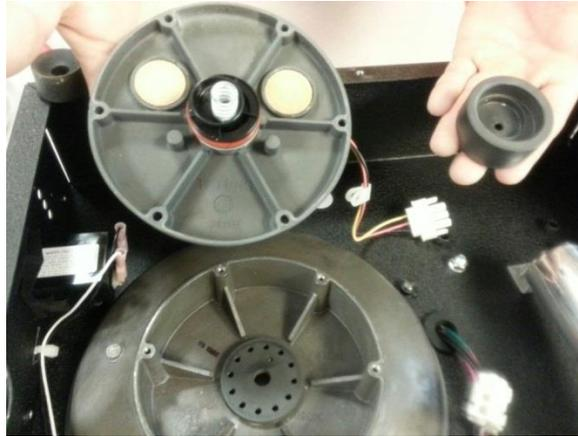
**Figure 5.15 ATF Motor Disassembled**
