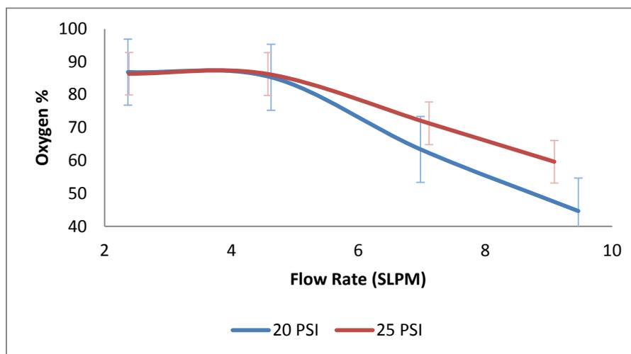
**Figure 5.4 Oxygen % Versus Flow Rate at 20 and 25 PSI**
