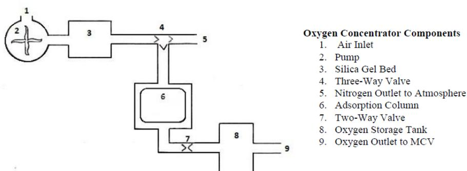
Figure 3.1 System Flow Diagram (20)
