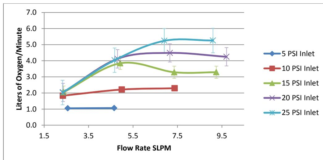
**Figure 6.4 Variable Inlet Pressure Oxygen Flow Rate**
